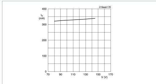
Fig 3. I<sub>out</sub> dependency as a function of AC supply voltage at 8 W output (120 V)
