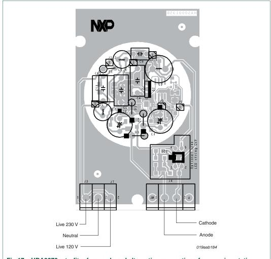
Fig 17. UBA3070 retrofit reference board alternative connections for experimentation
